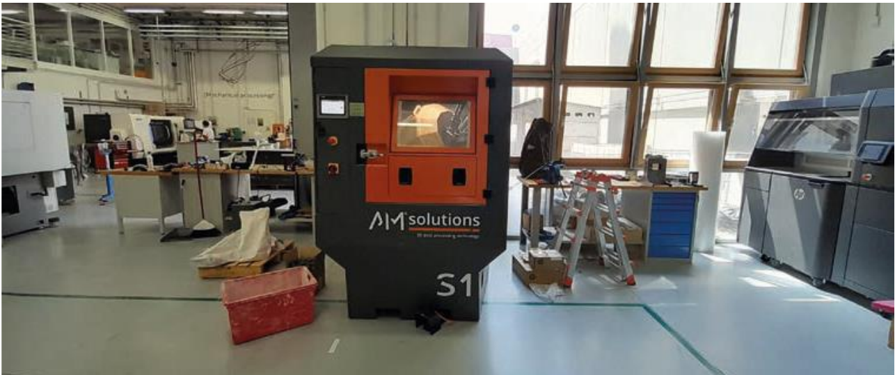
AM Solutions' Series 2 S1 machine is a multifunctional solution: it performs cleaning and surface finishing in one independent unit
